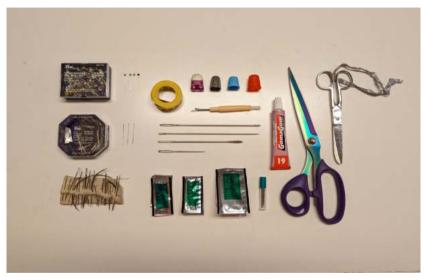
The sewing tools to be used are: Scissors, thick threads (30) and standard threads (120), thimbles, needles of different sizes, pins & fabric glue.
